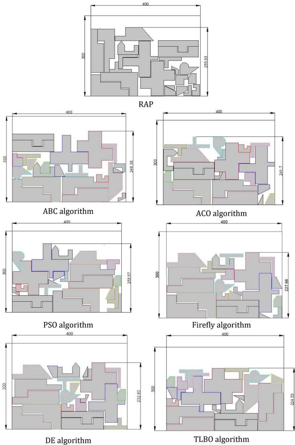
Figure 4. Optimal layouts for irregular shaped parts using different metaheuristics
