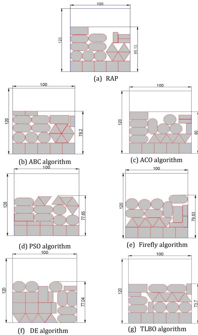
Figure 2. Optimal layouts for regular shaped parts using different metaheuristics
