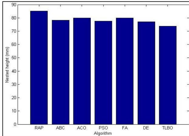
Figure 3. Comparison of nested heights for regular shaped parts
