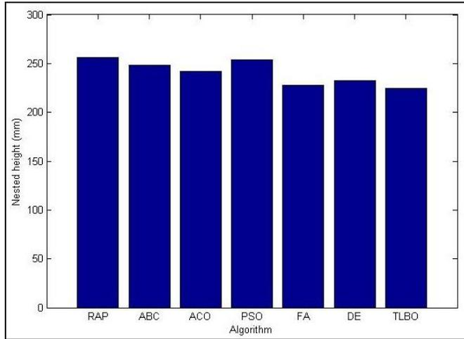
Figure 5. Comparison of nested heights for irregular shaped parts
